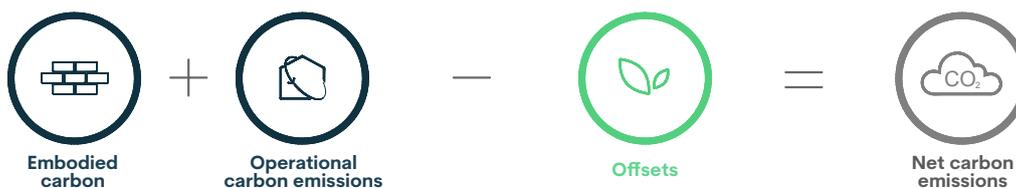
Figure 3: Calculation of the carbon emissions associated with a building.
