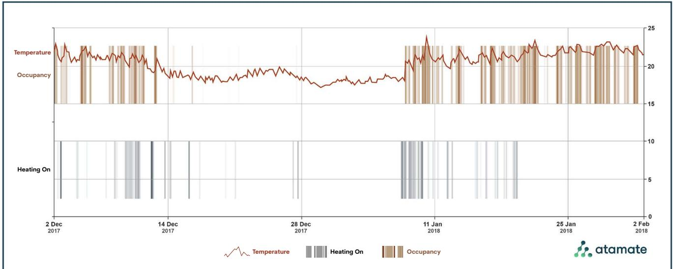
**Figure 13:** Occupancy-based electrical heating under atBOS controls in a single bedroom, showing the temperature dropping during a prolonged absence for the Christmas holidays but rapidly returning to the 21°C setpoint when the occupant returned.<sup>32</sup>
